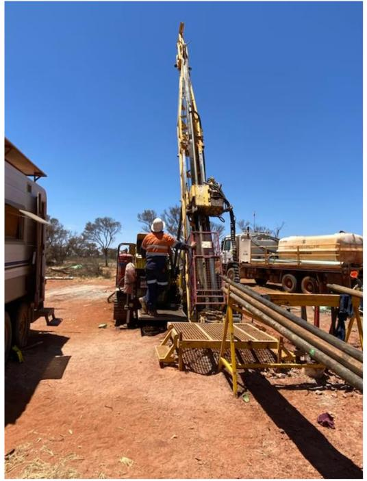
Figure 1 –Diamond Drill Rig operating at Abercromby Gold Project, Wiluna, WA
